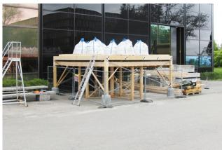
In recent years, the novel Timber Structures 3.0 technology (TS3) has been developed. This technology makes it possible to glue timber components made of solid, glulam or cross-laminated timber on the face side. This allows the creation of point-supported, multi-axis load-bearing slabs or folded structures of any shape and size.
